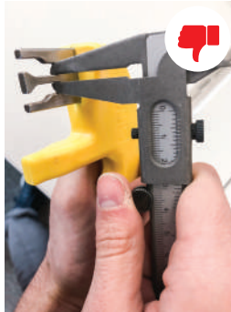
Key requires replacement
